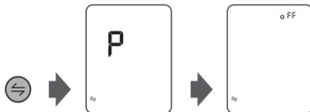
3. Press the [START/STOP] button to turn the monitor off.
